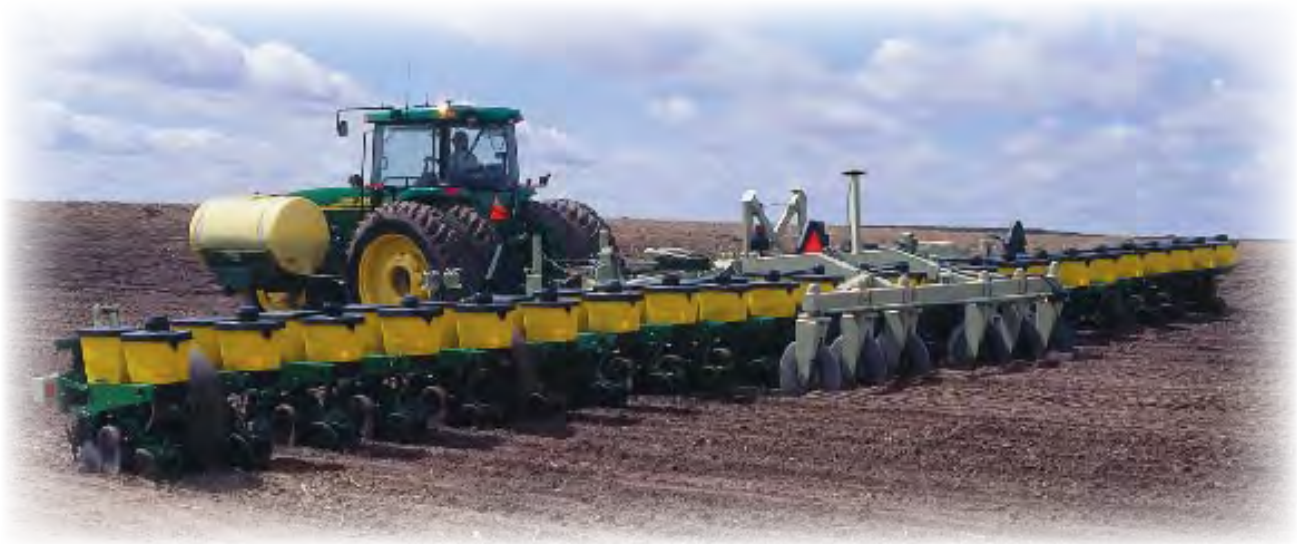
(6-Blade Tracker IV Guidance System mounted to a 1900 Series Planter Toolbar)
