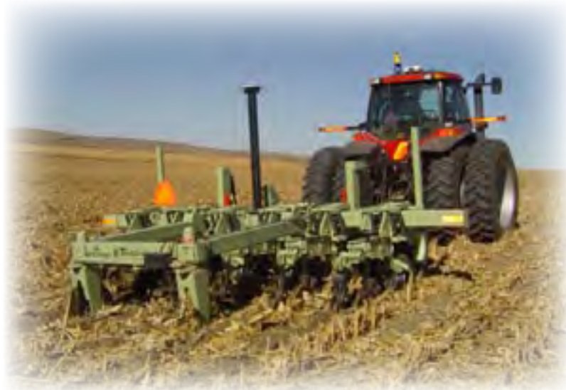
(2-Blade Tracker IV Guidance System mounted to a 6 row 30" Orthman 1tRIPr)
