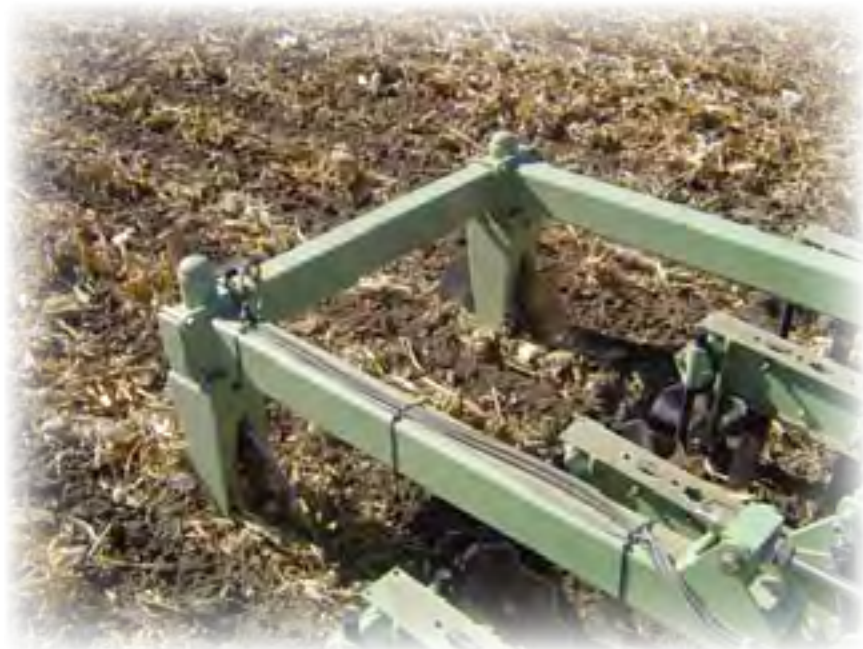
(2-Blade Tracker IV Guidance System mounted to a 6 row 30" Orthman 1tRIPr)
